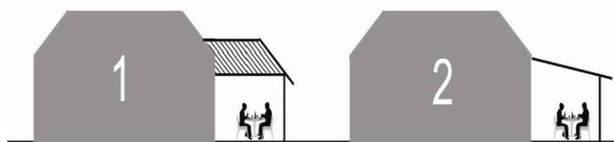
*The outdoor area to 1 has a bulkier roof form than 2*
