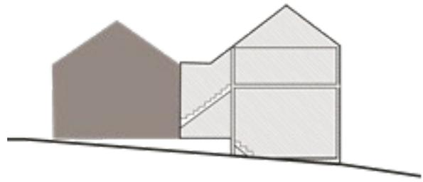
*Using a slope to reduce height of two storey rear additions*
