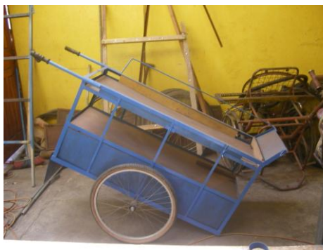
A steel-framed handcart manufactured at the Workshop
